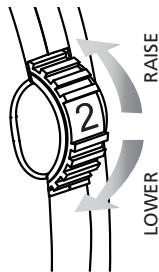
The volume control allows you to adjust the amplification of your hearing aid.
